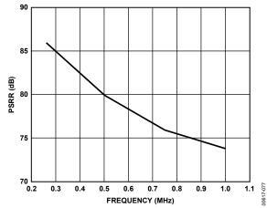
Figure 77. AVDD Power Supply Rejection Ratio vs. Frequency
