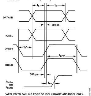
Figure 64. 5 V or 3.3 V Interleaved Mode Timing
