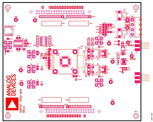
Figure 92. Assembly, Top Side
