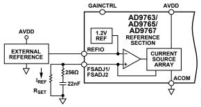
Figure 60. External Reference Configuration Gain Control Mode
