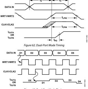
Figure 63. Dual-Port Mode Timing
