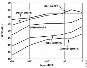
Figure 47. Single-Tone SFDR vs.  $A_{OUT} @ f_{OUT} = f_{CLK}/5$
