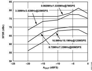
Figure 48. Dual-Tone SFDR vs. Aout @  $f_{OUT} = f_{CLK}/7$
