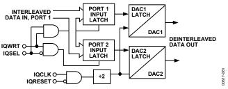
Figure 61. Latch Structure in Interleaved Mode
