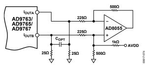
Figure 74. Single-Supply DC Differential-Coupled Circuit
