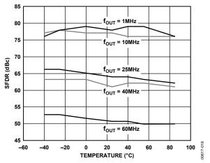
Figure 18. SFDR vs. Temperature @  $f_{CLK} = 125$  MSPS, 0 dBFS
