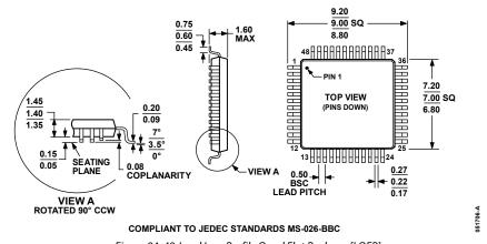
Figure 94. 48-Lead Low Profile Quad Flat Package [LQFP] (ST-48) Dimensions shown in millimeters
