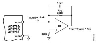
Figure 76. Unipolar Buffered Voltage Output
