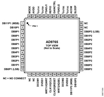
Figure 4. AD9765 Pin Configuration
