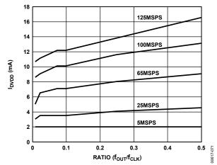
Figure 71. I<sub>DVDD</sub> vs. Ratio @ DVDD1 = DVDD2 = 3.3 V
