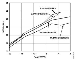
Figure 12. Single-Tone SFDR vs. Aout @  $f_{OUT} = f_{CLK}/11$
