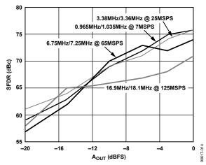
Figure 14. Dual-Tone SFDR vs.  $A_{OUT}$  @  $f_{OUT} = f_{CLK}/7$
