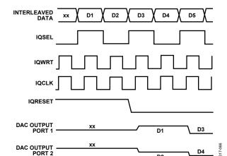
Figure 66. Interleaved Mode Timing
