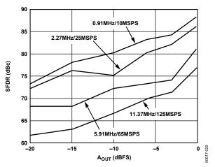
Figure 29. Single-Tone SFDR vs. Aout @  $f_{OUT} = f_{CLK}/11$
