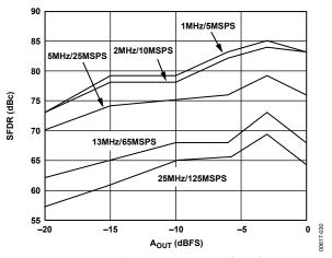
Figure 30. Single-Tone SFDR vs.  $A_{OUT} @ f_{OUT} = f_{CLK}/5$
