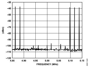
Figure 81. AD9765 Notch in Missing Bin at 5 MHz Is Down >60 dB (Peak Amplitude = 0 dBm)
