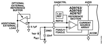
Figure 59. Internal Reference Configuration
