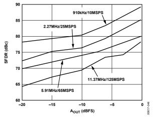
Figure 46. Single-Tone SFDR vs. Aout @  $f_{OUT} = f_{CLK}/11$
