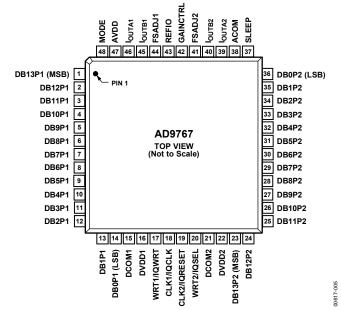
Figure 5. AD9767 Pin Configuration
