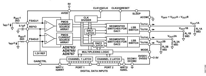
NOTES 1. IN THIS CONFIGURATION, THE 22nF CAPACITOR AND 256 $\Omega$  RESISTOR ARE NOT REQUIRED BECAUSE R<sub>SET</sub> =  $2k\Omega$ .
