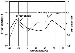
Figure 19. Gain and Offset Error vs. Temperature @  $f_{CLK} = 125 \text{ MSPS}$
