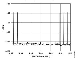
Figure 82. AD9767 Notch in Missing Bin at 5 MHz Is Down >60 dB (Peak Amplitude = 0 dBm)
