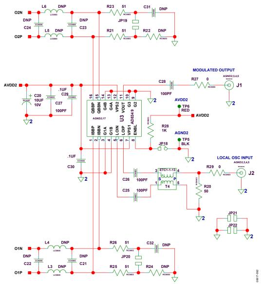
Figure 88. Modulator on AD9763/AD9765/AD9767 Evaluation Board
