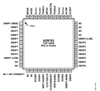
Figure 3. AD9763 Pin Configuration
