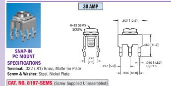
SEMS Screw Terminals provide quick and secure attachment of wire leads. SEMS screw has captivated, free spining lock washer, eliminated twisting of wire when tightening lead to terminal. Washer will rise with head of screw when unscrewed.
