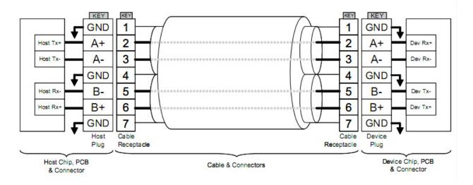
Figure 1-3 SATA Cable/Connector Connection Diagram
