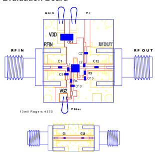
The above thru line can be provided to de-embed the losses of the evaluation board.
