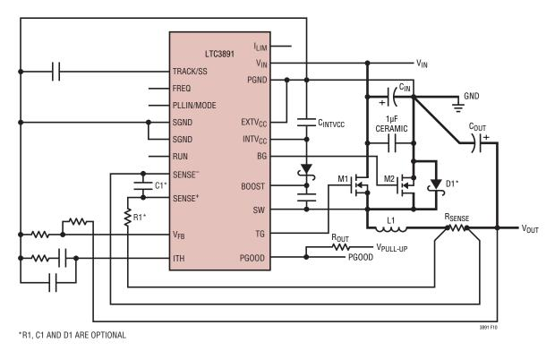
Figure 10. Recommended Printed Circuit Layout Diagram
