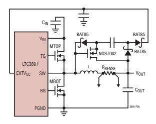
Figure 8. Capacitive Charge Pump for EXTV<sub>CC</sub>
