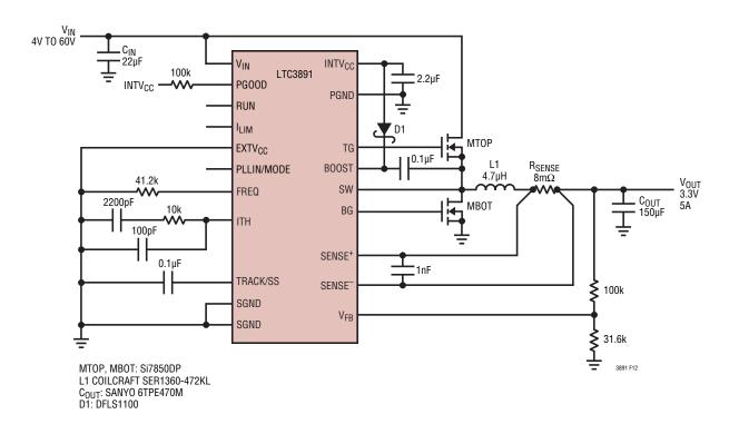
Figure 12. High Efficiency 3.3V Step-Down Converter
