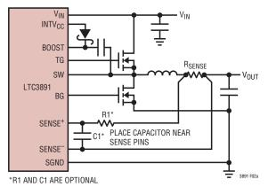
(2a) Using a Resistor to Sense Current
