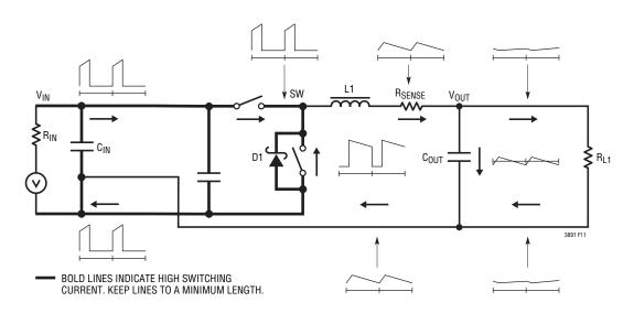
Figure 11. Branch Current Waveforms
