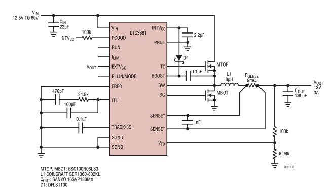
Figure 13. High Efficiency 12V Step-Down Converter
