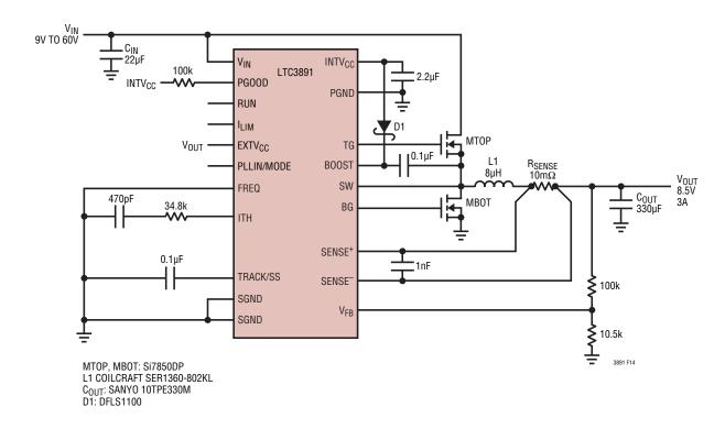
Figure 14. High Efficiency 8.5V Step-Down Converter
