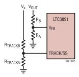
Figure 7. Using the TRACK/SS Pin for Tracking
