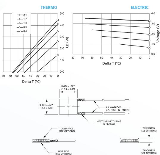
Ceramic Material: Alumina (Al<sub>2</sub>O<sub>3</sub>) Solder Construction: 138°C, Bismuth Tin (BiSn)
