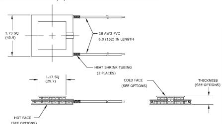
Ceramic Material: Alumina (Al<sub>2</sub>O<sub>3</sub>) Solder Construction: 138°C, Bismuth Tin (BiSn)
