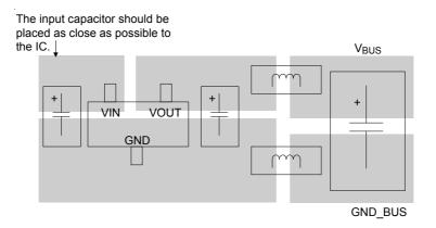
Figure 2. PCB Layout Guide
