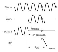
Figure 5. AC Disconnect Timing
