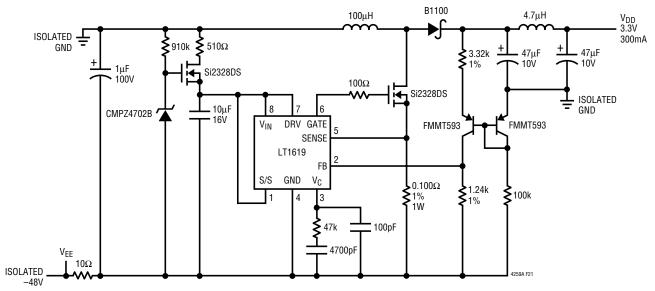
Figure 21. -48V to 3.3V Boost Converter
