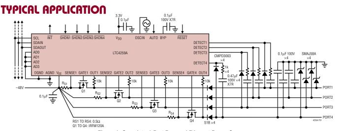
Figure 1. Complete 4-Port Powered Ethernet Power Source
