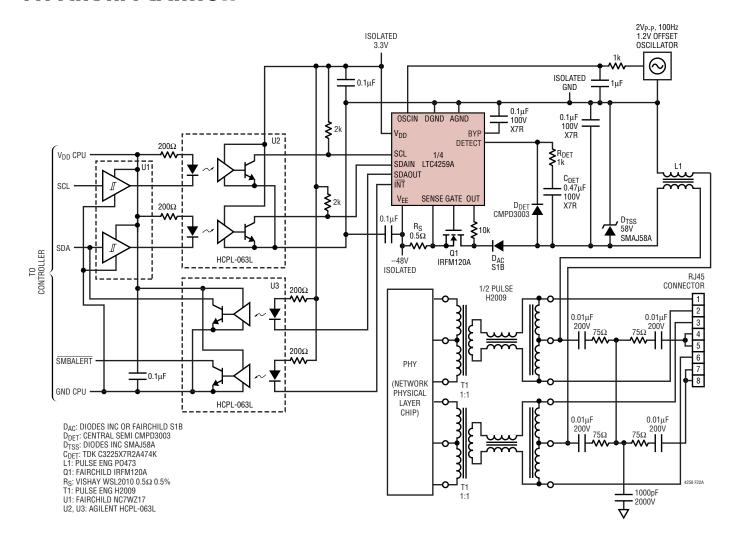
Figure 22. One Complete Isolated Powered Ethernet Port
