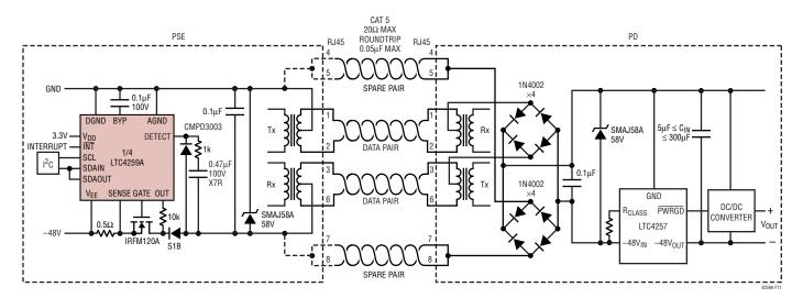
Figure 11. Power over Ethernet System Diagram
