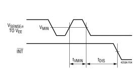
Figure 4. DC Disconnect Timing
