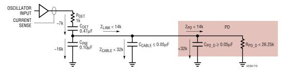
Figure 19. Simplified AC Disconnect Circuit with Impedances at 100Hz
