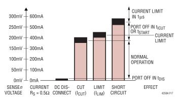
Figure 17. LTC4259A Current Sense and Limits
