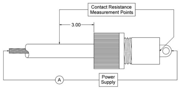
Figure 3 Contact Resistance Measurement Points
