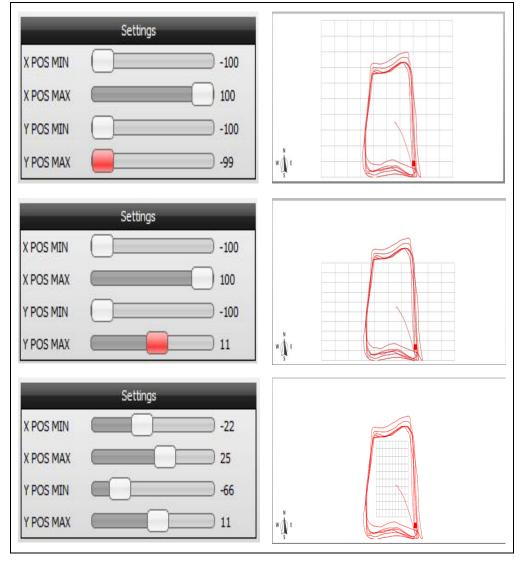
FIGURE 2-39: SENSING AREA – PARAMETER ADJUSTMENT
