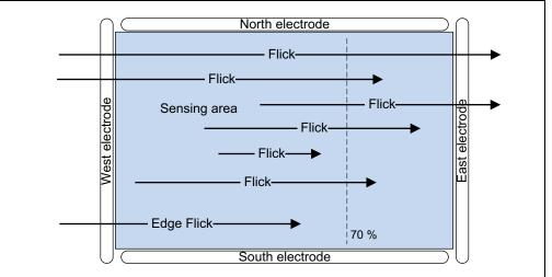
Colibri RTC supports the flick gestures listed in Table 2-1. The gestures can be individually enabled and disabled by checking and unchecking the respective check-boxes.
