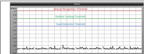
FIGURE 2-52: NOISE POWER – THRESHOLDS
