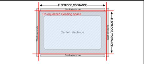
Adjust the electrode X and Y distances by using the respective slider (see Figure 2-26). For fine-tuning, click on the slider and use the arrow keys on your PC keyboard.
