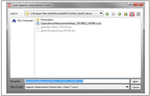
The Electrode Capacitance Measurement will automatically jump to the second step where a new measurement with auxiliary capacitors will be conducted. The first step measurement results will be displayed (see Figure 2-65). The user has to enter in the five soldered auxiliary capacitors values. Refer to "GestIC<sup>®</sup> Design Guide" (DS40001716) for more details.
