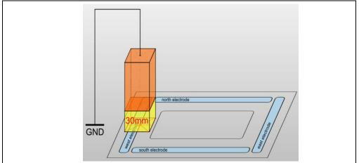
FIGURE 2-27: ELECTRODE WEIGHTING – ANIMATION BRICK POSITION
