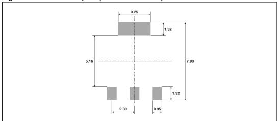
Figure 17. SOT-223 footprint (dimensions in mm)t
