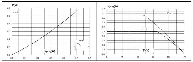
Figure 3. Average and D.C. on-state current versus ambient temperature (epoxy printed circuit board FR4, copper thickness = 35  $\mu$ m,  $S_{CU}$  = 0.5 cm<sup>2</sup>) (TO-92)
