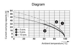
Derating curve for: DFK-PC 5/...-ST-7,62 with PC 5/...-ST-7,62 Conductor cross section = 6 mm<sup>2</sup>
