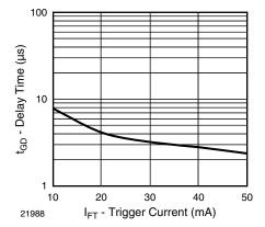
Fig. 9 - Trigger Current vs. Delay Time
