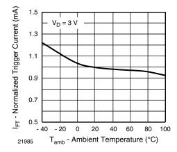
Fig. 6 - Normalized Trigger Current vs. Ambient Temperature
