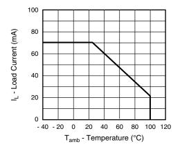
Fig. 1 - Recommended Operating Condition
