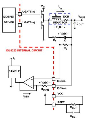
FIGURE 21. DCR SENSING CONFIGURATION
