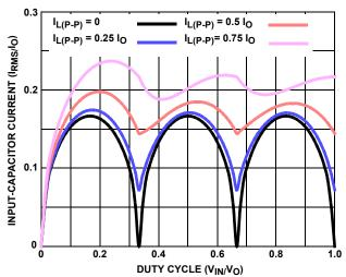
FIGURE 27. NORMALIZED INPUT-CAPACITOR RMS **CURRENT FOR 3-PHASE CONVERTER**
