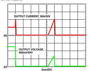
FIGURE 14. OVERCURRENT BEHAVIOR IN HICCUP MODE
