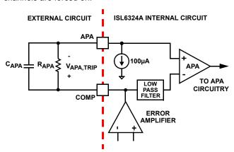
FIGURE 3. ADAPTIVE PHASE ALIGNMENT DETECTION
