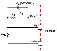
FIGURE 23. COMPENSATION CONFIGURATION FOR LOAD-LINE REGULATED ISL6324A CIRCUIT
