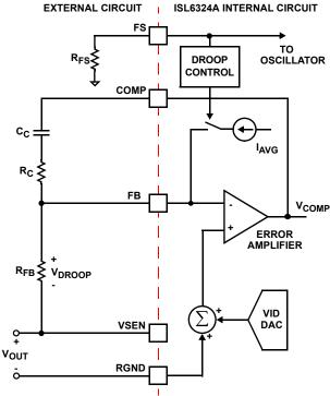
FIGURE 8. OUTPUT VOLTAGE AND LOAD-LINE REGULATION
