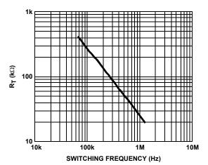
FIGURE 25. RT vs SWITCHING FREQUENCY
