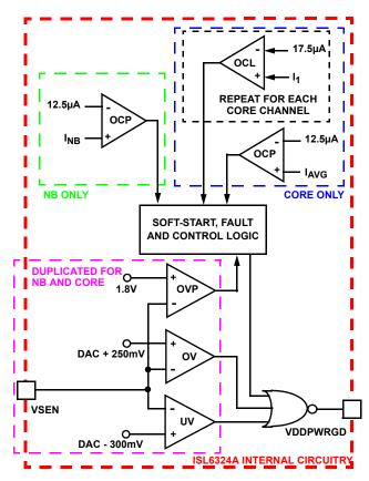
FIGURE 13. POWER-GOOD AND PROTECTION CIRCUITRY
