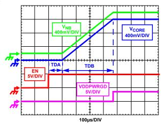
FIGURE 11. SOFT-START WAVEFORMS
