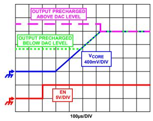
FIGURE 12. SOFT-START WAVEFORMS FOR ISL6324A-BASED MULTI-PHASE CONVERTER
