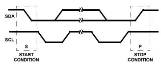
FIGURE 16. START AND STOP WAVEFORMS
