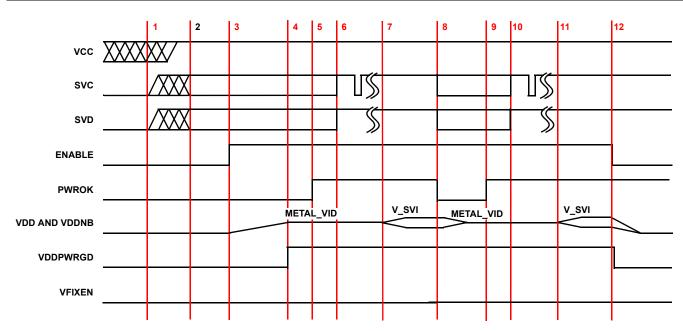
FIGURE 7. SVI INTERFACE TIMING DIAGRAM: TYPICAL PRE-PWROK METAL VID START-UP
