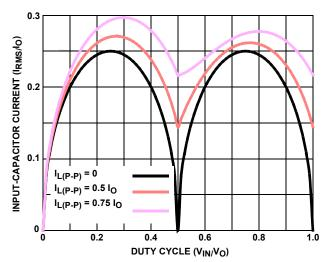
FIGURE 28. NORMALIZED INPUT-CAPACITOR RMS **CURRENT FOR 2-PHASE CONVERTER**
