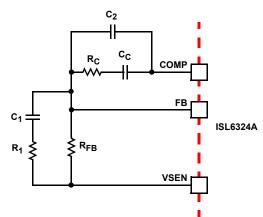
FIGURE 24. COMPENSATION CIRCUIT WITHOUT LOAD-LINE REGULATION
