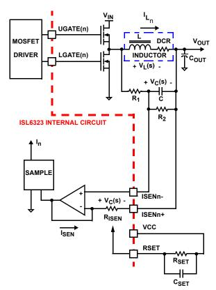
FIGURE 5. INDUCTOR DCR CURRENT SENSING CONFIGURATION
