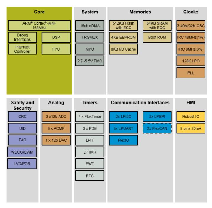
Figure 1. Kinetis KE1xF512 family block diagram
