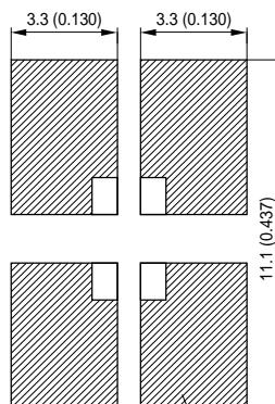
Cu Fläche /  $\geq 16 \text{ mm}^2$  per pad
