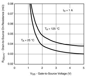
**On-Resistance vs. Gate-to-Source Voltage**
