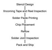
FIGURE 5. SMT Assembly Process Flow
