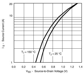
Source-Drain Diode Forward Voltage
