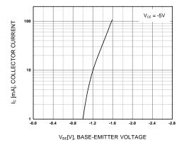
Figure 3. Base-Emitter On Voltage
