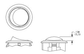
$\mbox{NOTE:}\ \mbox{J3}$  actuator available with the combination of 7 & 8 lamp ratings and CR102 switch function only.
