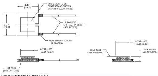
Ceramic Material: Alumina ( $Al_2O_3$ ) Solder Construction: 138°C, Bismuth Tin (BiSn)
