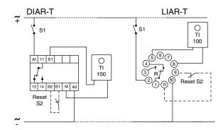
Note: Upon energization of the current control IAR.T Series Relay, the time delay, which is adjustable from .1 to 10 seconds, inhibits the output relay during start-up periods. The delay time is adjustable via a potentiometer located on the side of the case. For additional current transformer see "Accessories" section: L595 Series.
