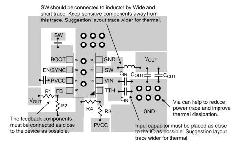
Figure 6. PCB Layout Guide
