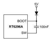
Figure 2. External Bootstrap Diode
