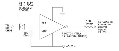
Simple driver using inexpensive standard logic ICs provides fast switching using minimum DC current. \* Recommended value to suppress unwanted RF signals at V1 - V6 control lines.
