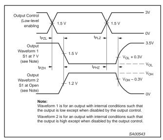
Waveform 2. 3-State Output Enable and Disable Times
