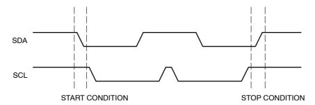
Figure 4. Start/Stop Timing
