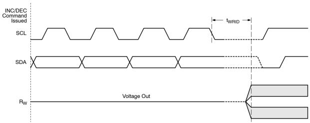
Figure 13. Increment/Decrement Timing Limits
