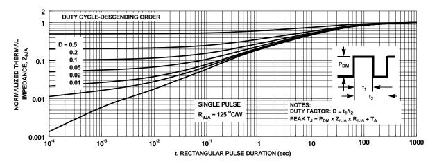
Figure 13. Junction-to-Ambient Transient Thermal Response Curve
