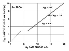
Figure 7. Gate Charge Characteristics
