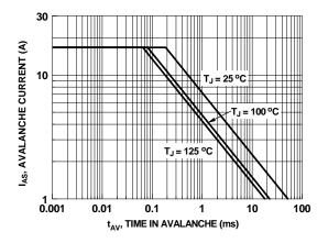
Figure 9. Unclamped Inductive Switching Capability
