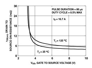
Figure 4. On-Resistance vs Gate to Source Voltage
