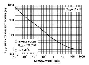
Figure 12. Single Pulse Maximum Power Dissipation
