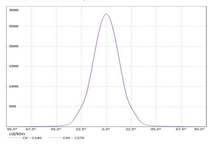
Luminaire: LEDiL Oy CN13108\_LENA-M-DL\_(Soleriq\_E30) Eff.78% Lamps: 1 x Osram Soleriq E30 (1240lm@250mA)
