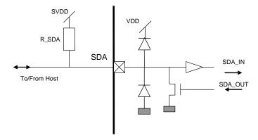
Figure 30: SDA Simplified Diagram
