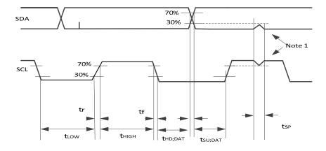
Figure 4: I2C Data Timing
