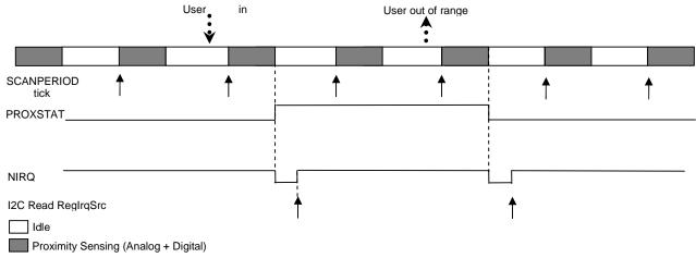
Figure 20: Proximity Sensing Host Operation (ReglrgMsk[6:3] = 1100)
