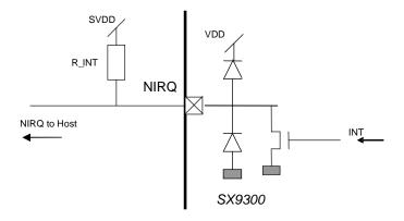
Figure 28: NIRQ Output Simplified Diagram
