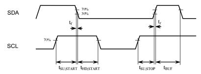
Figure 3: I2C Start and Stop Timing
