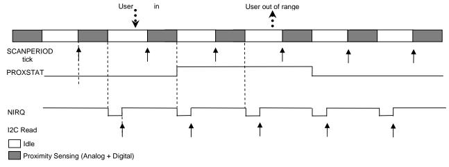
Figure 21: Proximity Sensing Host Operation (ReglrqMsk[6:3] = 0001)
