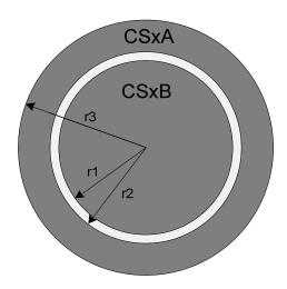
Figure 22: Typical Smart SAR Capacitive Sensor
