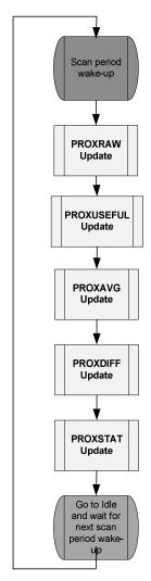
Figure 13: Digital Processing Sequencing
