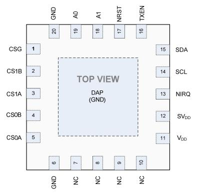
Figure 1: Pin Diagram
