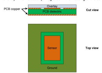
Figure 7: Typical Capacitive Sensing Implementation
