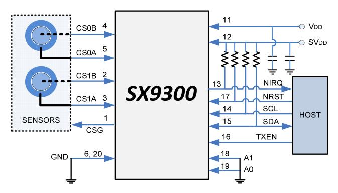
Figure 31: Typical Application Circuit
