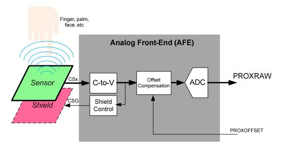
Figure 9: Analog Front-End Block Diagram
