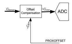
Figure 10: Offset Compensation Block Diagram
