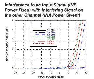
Interference to an Input Signal (INA Power Fixed) with Interfering Signal on the other Channel (INB Power Swept)
