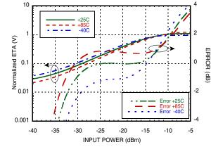
ETA vs. Pin with CW @ 1900 MHz
