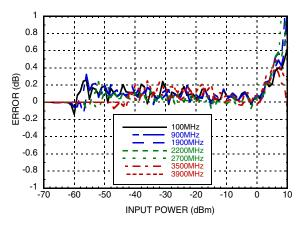
RMSA vs. Pin w/ CW & WCDMA 4 Carrier @ 1900 MHz & -40°C <sup>[1] [2]</sup>
