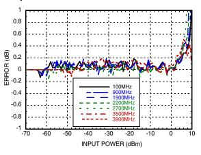
RMSA vs. Pin w/ CW & WCDMA 4 Carrier @ 1900MHz & +85°C <sup>[1] [2]</sup>
