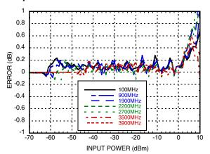
RMSB vs. Pin w/ CW & WCDMA 4 Carrier @ 1900 MHz & -40°C <sup>[1] [2]</sup>
