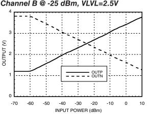
With the channels of HMC1030LP5E having very low mismatch, and located on the same die, the channel outputs RMSA and RMSB track very closely over temperature. The difference operation also allows the OUTP and OUTN to reject common-mode changes in channels A and B.
