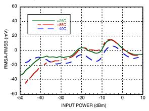
RMSA-RMSB, Channel Matching vs. Pin over Temperature @ 2200 MHz <sup>[2] [3]</sup>
