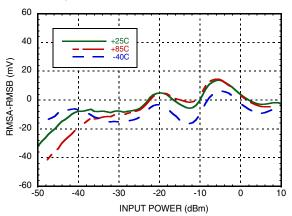
RMSA-RMSB, Channel Matching vs. Pin over Temperature @ 1900 MHz<sup>[2][3]</sup>
