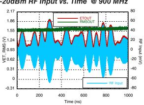
VRMSA & VETA & WCDMA 4 Carrier with -20dBm RF Input vs. Time @ 900 MHz
