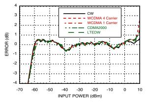
RMSB vs. Pin with Different Modulations @ 1900 MHz<sup>[1]</sup>
