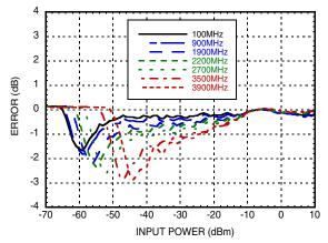
RMSB Error vs. Pin with WCDMA 4 Carrier @ -40°C wrt +25°C Response <sup>[1] [2]</sup>
