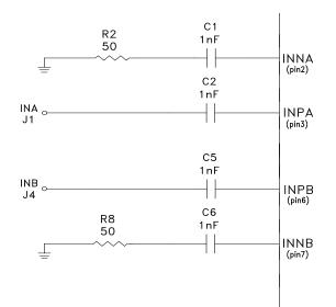
Note that the provided single-ended input interface covers the whole operating spectrum of the HMC1030LP5E and does not require matching tuning for different frequencies. The performance of the HMC1030LP5E at different frequencies is shown below:
