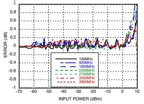
RMSA-RMSB, Channel Matching vs. Pin over Temperature @ 900 MHz <sup>[2] [3]</sup>
