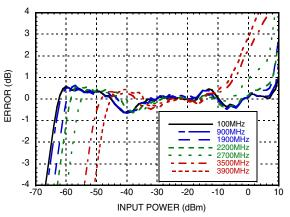
RMSA Error vs. Pin with WCDMA 4 Carrier @ +85°C wrt +25°C Response <sup>[1] [2]</sup>
