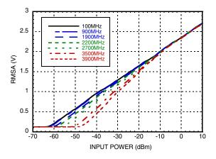
RMSA Error vs. Pin with CW @ +25°C <sup>[1] [2]</sup>
