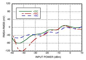
Interference to an Input Signal (INB Power Fixed) with Interfering Signal on the other Channel (INA Power Swept) <sup>[1]</sup>
