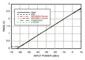
RMSA Error vs. Pin with Different Modulations @ 1900 MHz<sup>[1]</sup>
