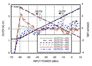
OUT [P,N] & Error vs. Pin @ 2200 MHz [1][2]
