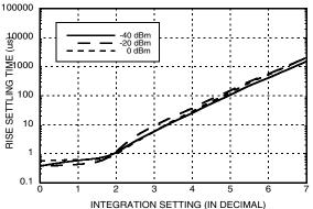
[1] Measured from 10% to 90% [2] Measured from RF switching edge to 1dB (input referred) settling of RMSOUT.
