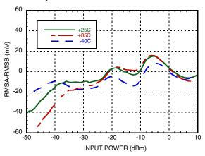
RMSA-RMSB, Channel Matching vs. Pin over Temperature @ 2700 MHz <sup>[2] [3]</sup>
