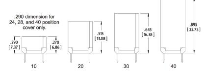
ALL DIMENSIONS: INCHES [MILLIMETERS] ALL TOLERANCES: ±0.005 [0.13] UNLESS OTHERWISE SPECIFIED FOR MATING DIP HEADER, SEE DATA SHEET 12032 **CONSULT FACTORY FOR OTHER SIZES AND CONFIGURATIONS**
