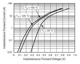
Fig. 3 - Typical Instantaneous Forward Characteristics
