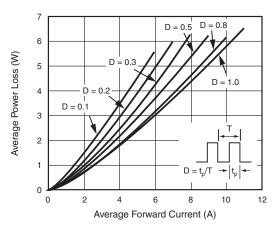
Fig. 2 - Forward Power Loss Characteristics
