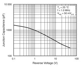
Fig. 5 - Typical Junction Capacitance
