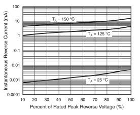
Fig. 4 - Typical Reverse Leakage Characteristics
