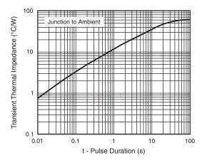
Fig. 6 - Typical Transient Thermal Impedance
