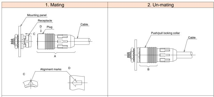
When mounting, smooth mating will be achieved by holding plug in any are "A" and aligning the arrow of the plug with that of the receptacle, then pushing the plug straight in.
