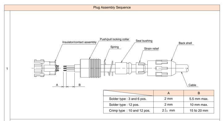
Thread the back shell, strain relief, seal bushing, spring and push/pull locking collar over the cable as shown above.
