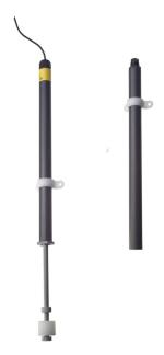
A vertical float switch, with either normally open or normally closed switch action, permanently joined to a 300mm PVC tube. This provides a switch, whose overall switching depth can be varied between 123mm and 423mm
