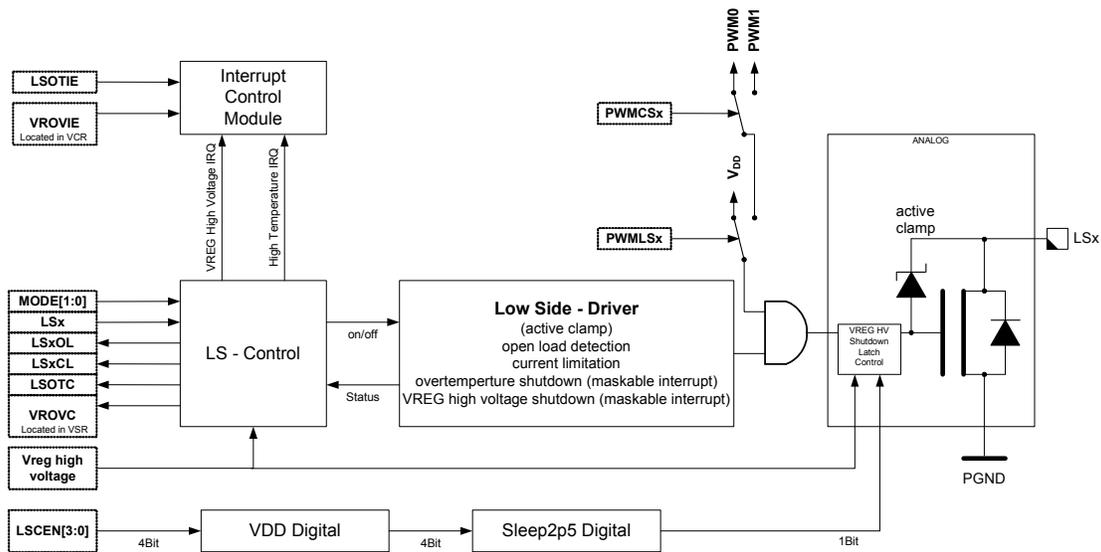
Figure 1. Low Side Block Diagram
