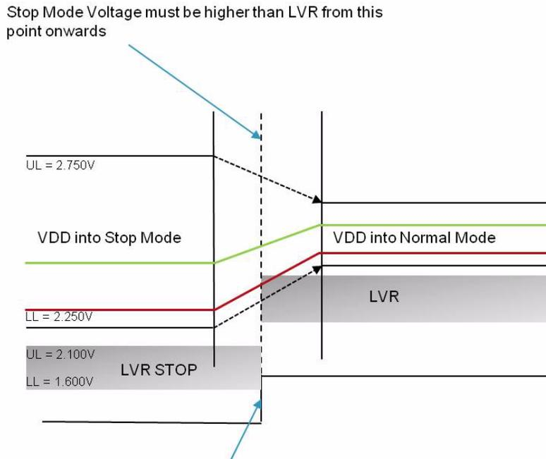
**Figure 2. Stop mode to Normal mode Transition**
