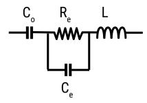
$C_{_{\alpha}}$  = Aluminum oxide capacitance (surface and thickness of the dielectric)
