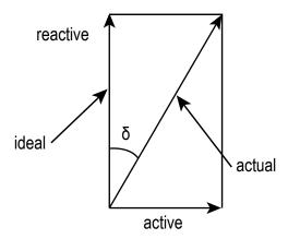
Tan  $\delta$  is measured with the same set-up used for the series capacitance ESC. tan  $\delta$  =  $\omega$  x ESC x ESR where:
