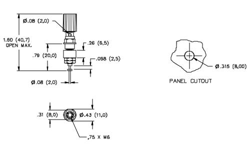
Recommended Maximuml Panel Thickness: .12" (3,0mm)
