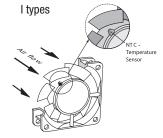
The temperature sensor (NTC resistor) for controlling the motor speed is positioned in the fan hub directly in the air flow.
