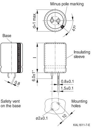
Safety vent on the base ø2±0.1 ø2.5 min. Snap-in terminals, length (6.0 ±1) mm. Also available in a shorter version with a length of (4.5 - 1) mm. PET insulation is marked with "PET" on the sleeve.
