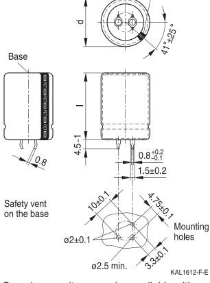
Snap-in capacitors are also available with 3 terminals (length (4.5 - 1) mm). PET insulation is marked with "PET" on the sleeve.
