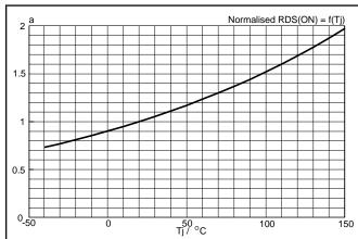
Fig.5. Normalised drain-source on-state resistance.  $a = R_{DS(ON)}/R_{DS(ON)}25^{\circ}C = f(T_i); I_D = 100 \text{ mA}; V_{IS} = 4.4 \text{ V}$
