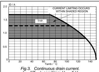
$I_D = f(T_{amb})$ ; condition:  $V_{IS} = 5 \text{ V}$
