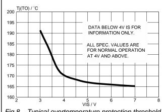
Fig.8. Typical overtemperature protection threshold.  $T_{i(TO)} = f(V_{IS})$
