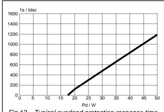
Fig.13. Typical overload protection response time.  $1/t_{dsc} = f(P_D); \ V_{IS} \ge 4 \ V, \ T_j \le 125 \ C.$
