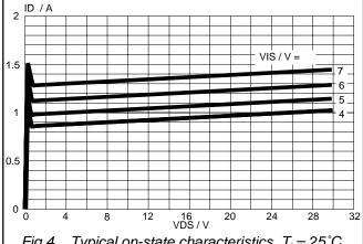
Fig.4. Typical on-state characteristics,  $T_j = 25$  °C.  $I_D = f(V_{DS})$ ; parameter  $V_{IS}$ ;  $t_p = 300 \, \mu s$
