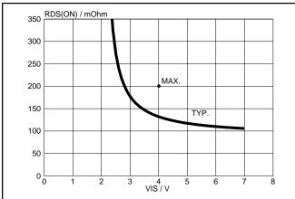
Fig.6. Typical on-state resistance,  $T_j = 25$  °C.  $R_{DS(ON)} = f(V_{IS})$ ; conditions:  $I_D = 100$  mA,  $t_p = 300$   $\mu s$
