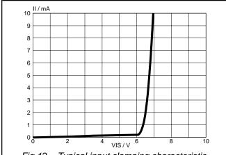
Fig.12. Typical input clamping characteristic.  $I_l = f(V_{lS})$ ; normal operation,  $T_j = 25$ °C.
