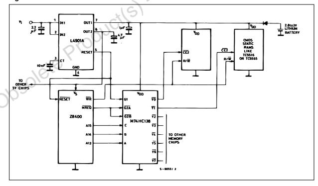
disable the  $\mu P$  and, through the address decoder M74HC138, to ensure that the RAMS are disabled as soon as the main supply starts to fall.
