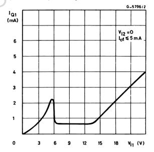
Figure 9: Total Quiescent Current versus Input Voltage
