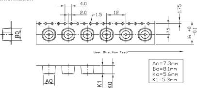
Parts packaged on 13" Diameter reel, 1,000 parts per reel.
