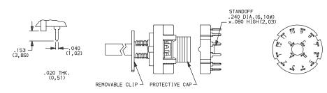
**NOTE:** Switches with 'C' or 'MC' terminations have additional terminal no. 9 as switch support only. This terminal is not connected electrically inside switch. Solder and clean switch base on PC board with other components, then snap on housing/actuator assembly. See page K-7 for installation instructions.
